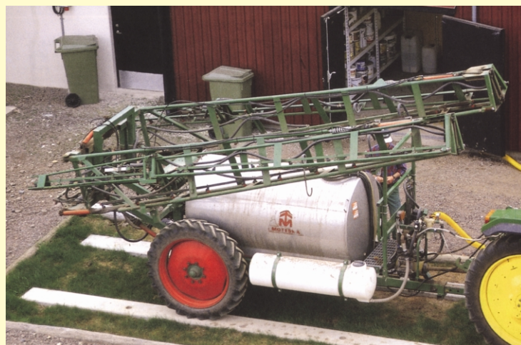
A safe place for filling and cleaning of the sprayer is one of the actions against potential contamination of water that is suggested in the campaign Safe Pesticide Use . In this case a 60 cm deep biobed - containing chopped straw, peat and topsoil - is used. Photo: Per Emgardsson/LandBild
